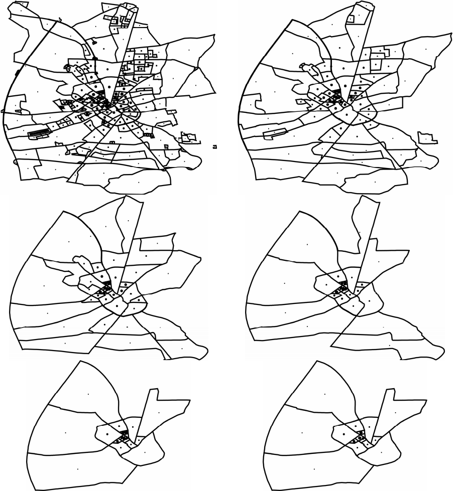
Fig. 5. Aggregation of road polygons in an iterative process using strokes as border lines
