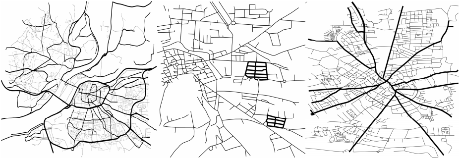
Fig. 1. Strokes (left), grids (middle) and star (right) detected in different data sets (Heinzle et al., 2005)
